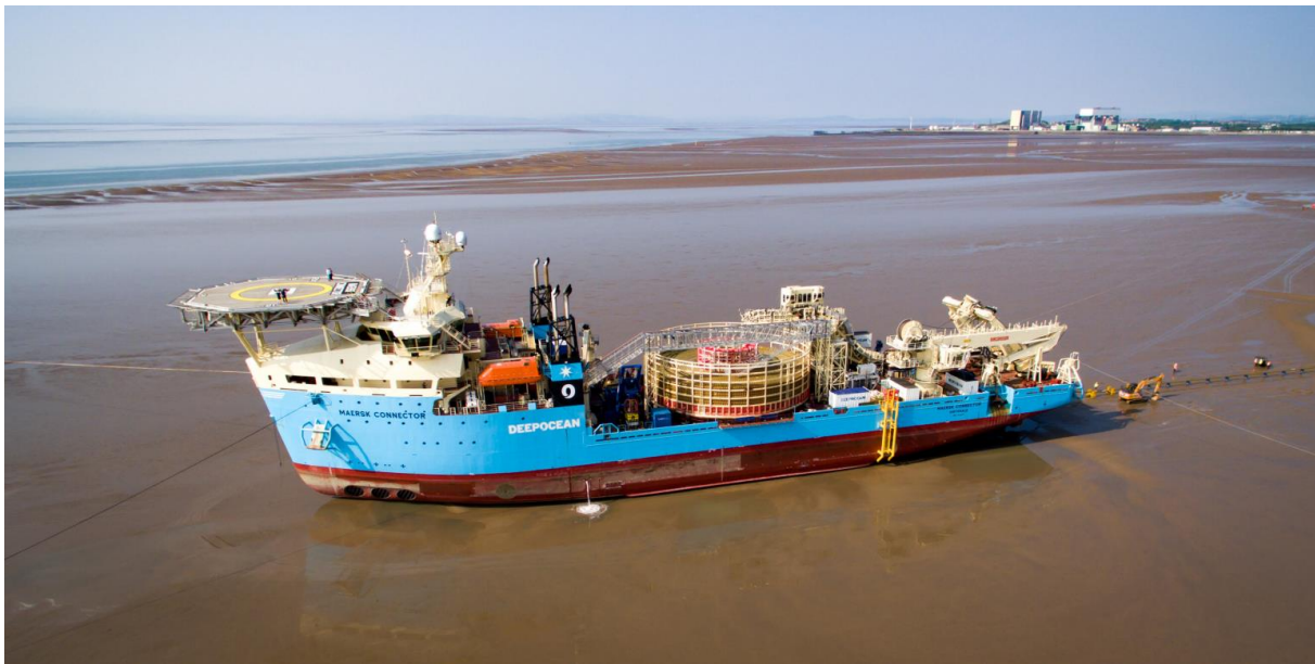
Figure 27: Delta Subsea's Connector performing a beached cable landing
